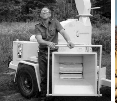
The year was 1983. The very first Bandit chipper was built in a 6,000 square-foot converted repair shop, with the assistance of just six employees. That first machine was the Model 100 Brush Bandit—a 12-inch capacity, hand-fed disc-style chipper (shown here).
