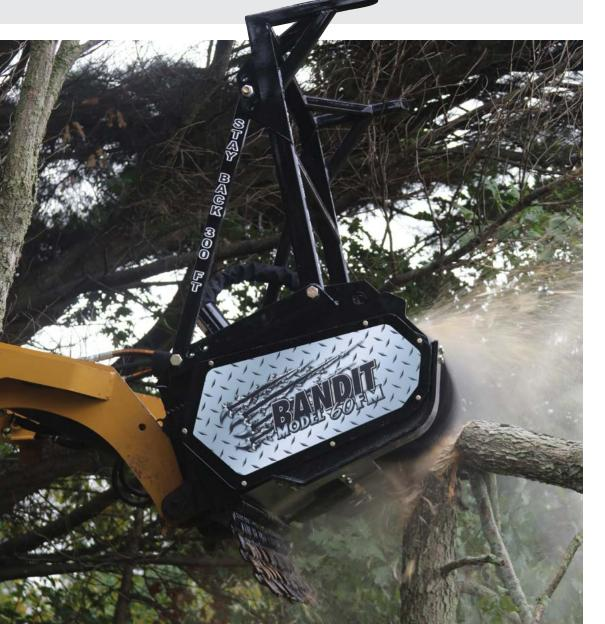
The **exclusive anvil** that is standard on every Bandit head acts as a second cutting surface, producing the best end product on the first pass. This **improves productivity** and **reduces fuel consumption**, while also preventing material from jamming the drum, a common problem among competitor's equipment.
