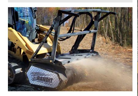
The strength of Bandit's forestry mulching attachments is their ease of use. They attach quickly via a quick attach plate and are operated by the loader's existing hydraulic systems. That means it takes only a few moments to attach either the Model 60FM or the Model 72FM and get to work. The loader powers a single variable speed hydraulic motor on the mulching head, giving the mulchers impressive grinding power with very simple maintenance.
