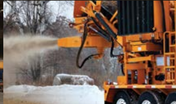
The Beast is being used to size, hay, straw, cane grass, switch grass and mescanthis to fuel biomass boilers in many parts of the world.
