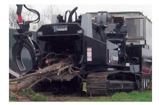
**VERSATILE – ON THE GO** This towable chipper is also available as a self-propelled machine riding on a CAT steel-track undercarriage.
